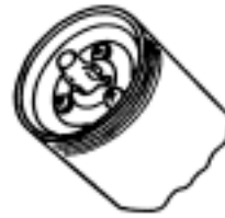
UNLOCKED LUGS PARRALLEL TO SLOT
